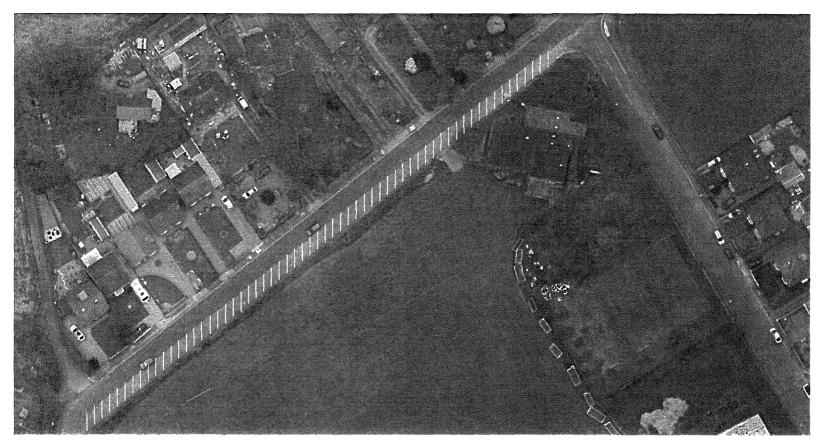
Simulated illustration of parking space layout for users of the sports ground. A 45° herringbone parking space would require a speed controlled access/egress lane width of 3.8m to safely use the allocated parking spaces. In this scenario we only have the public highway.
