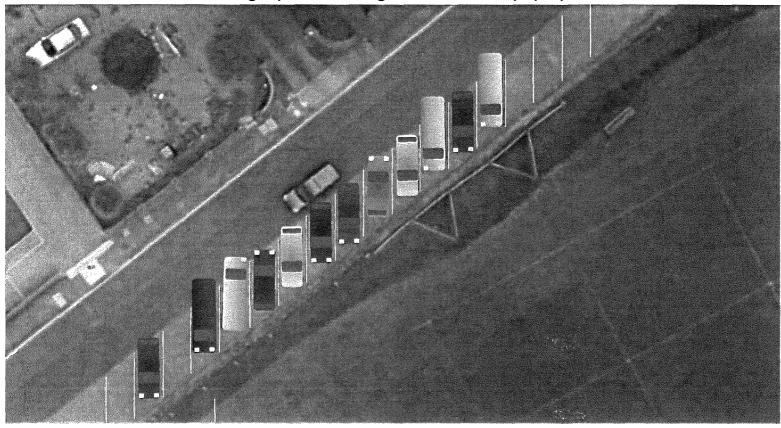
As you can see from the simulated illustration, the recently marked parking spaces do not fully contain vehicles from overhanging into the public highway. Furthermore on exiting the parking spaces, vehicles have little to no sighting distance to oncoming traffic and regularly reverse blind into the line of traffic. The standard visibility splay for an new access onto 30mph road is 43m (or 25m at 20mph), these do not meet current guidelines for Nottinghamshire.
