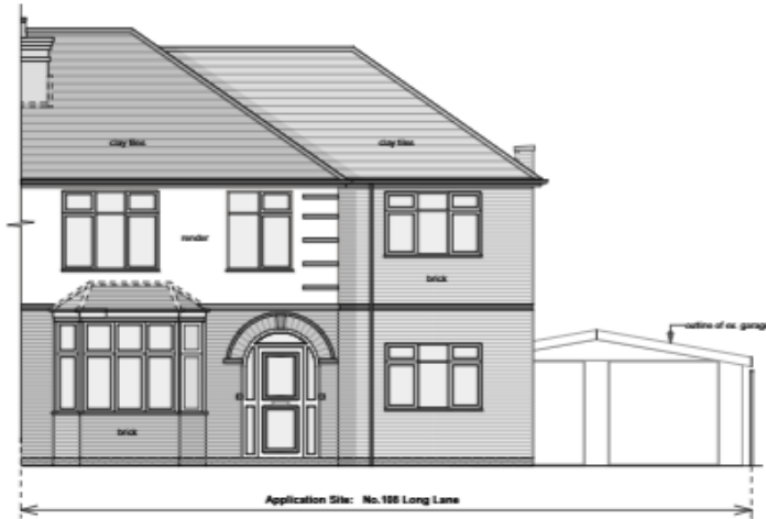
① Front Elevation (Along Long Lane) Scale: 1:100
